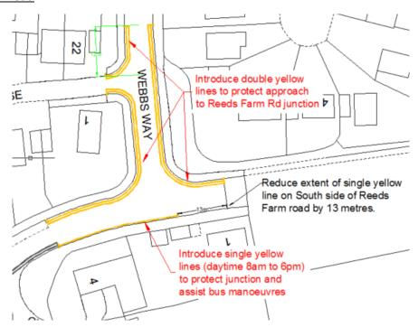
Reduce the extent of SYL to the south of Reeds Farm Road by 13 metres to protect accesses. This is reduction is not expected to affect the visibility of the junction as the road acts like a bend with a dead end to the east of the road.
